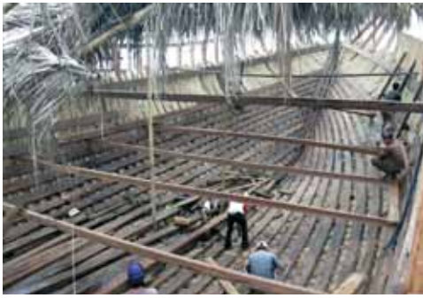
Fig. 7 A phinisi boat is under construction, Day 3 [Gb. 7 Konstruksi perahu Phinisi, hari ke-3]
